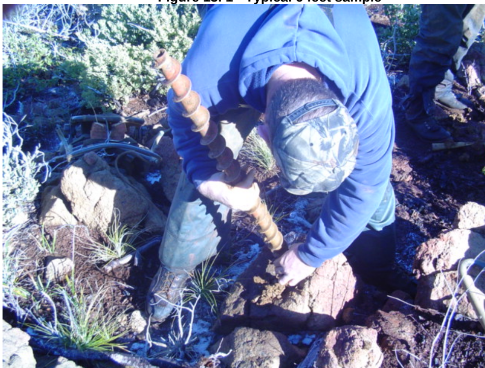
Figure 13. 2 - Systematic rod cleaning between sampling runs
