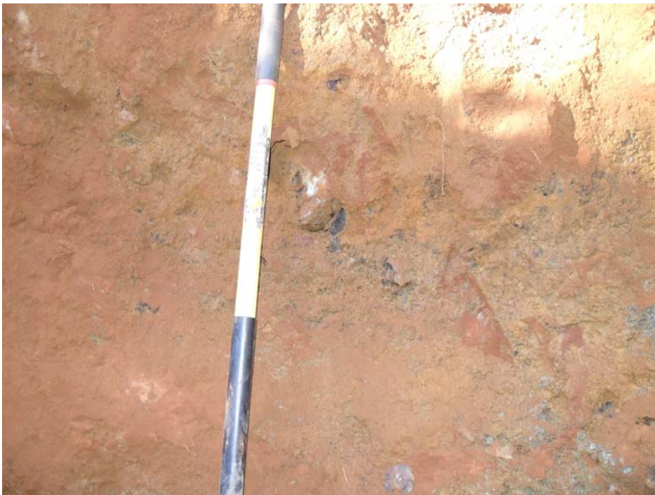
Saproplitic horizon –trench no. 1
