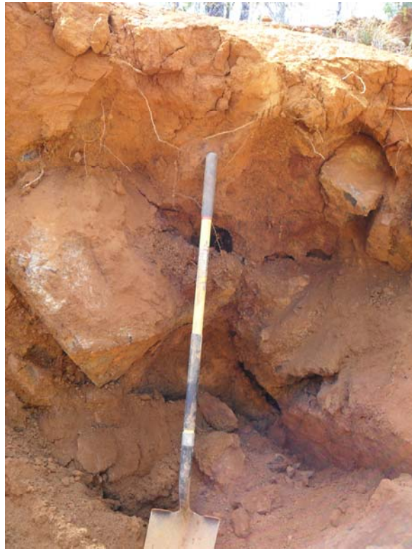
Figure 12. 5 - Typical soil and corestone profile (trench no. 4)
