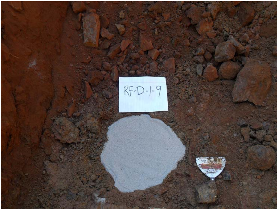
Density sample – trench no. 1, 9 ft (the sand is used to measure the volume)
