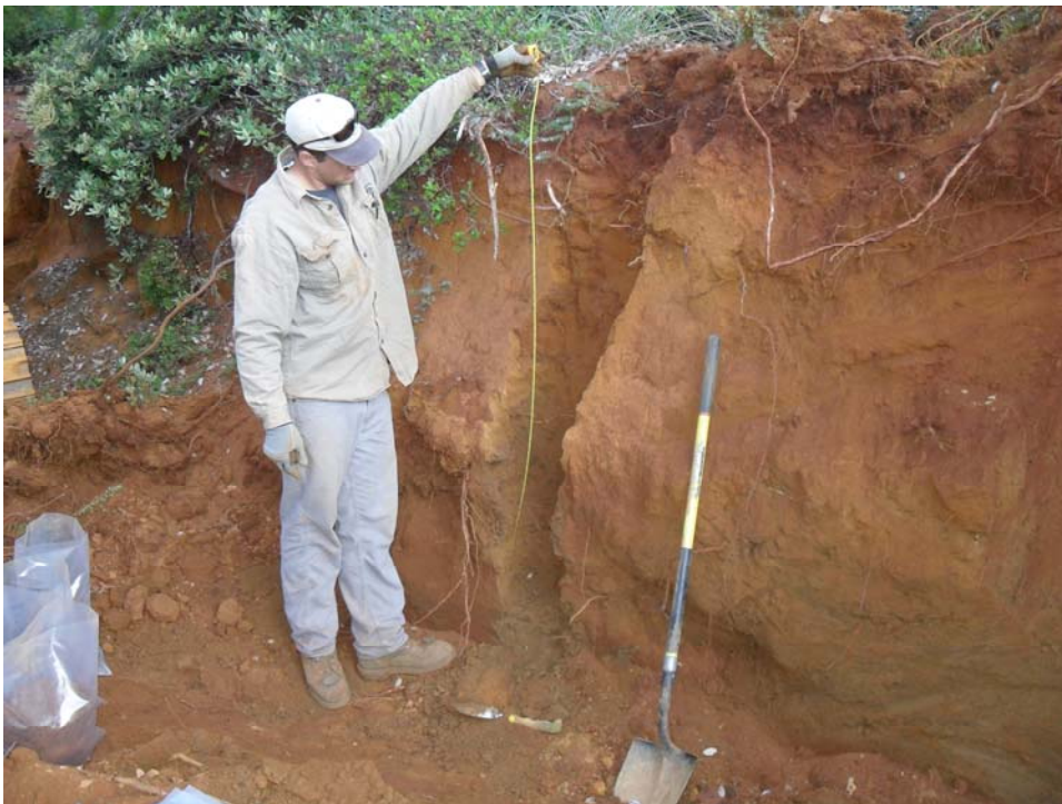
Channel sample – trench no.3
